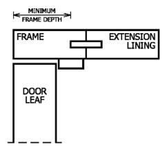
HEAD/JAMB JOINT: Mortice and tenon, or half-lapped joint, head twice screwed to each jamb.
