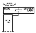
In scenarios where the face of the frame, and the door, are flush with the face of the wall, architraves may be 'loose' (i.e. pin-fixed), but are optional, subject to adequate fire-stopping; (See Section 3.9 regarding wall/frame gaps).
